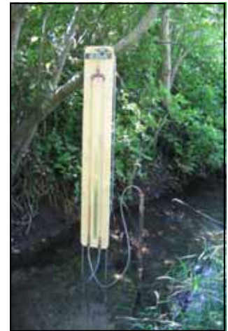
Piezometer with manometer board
