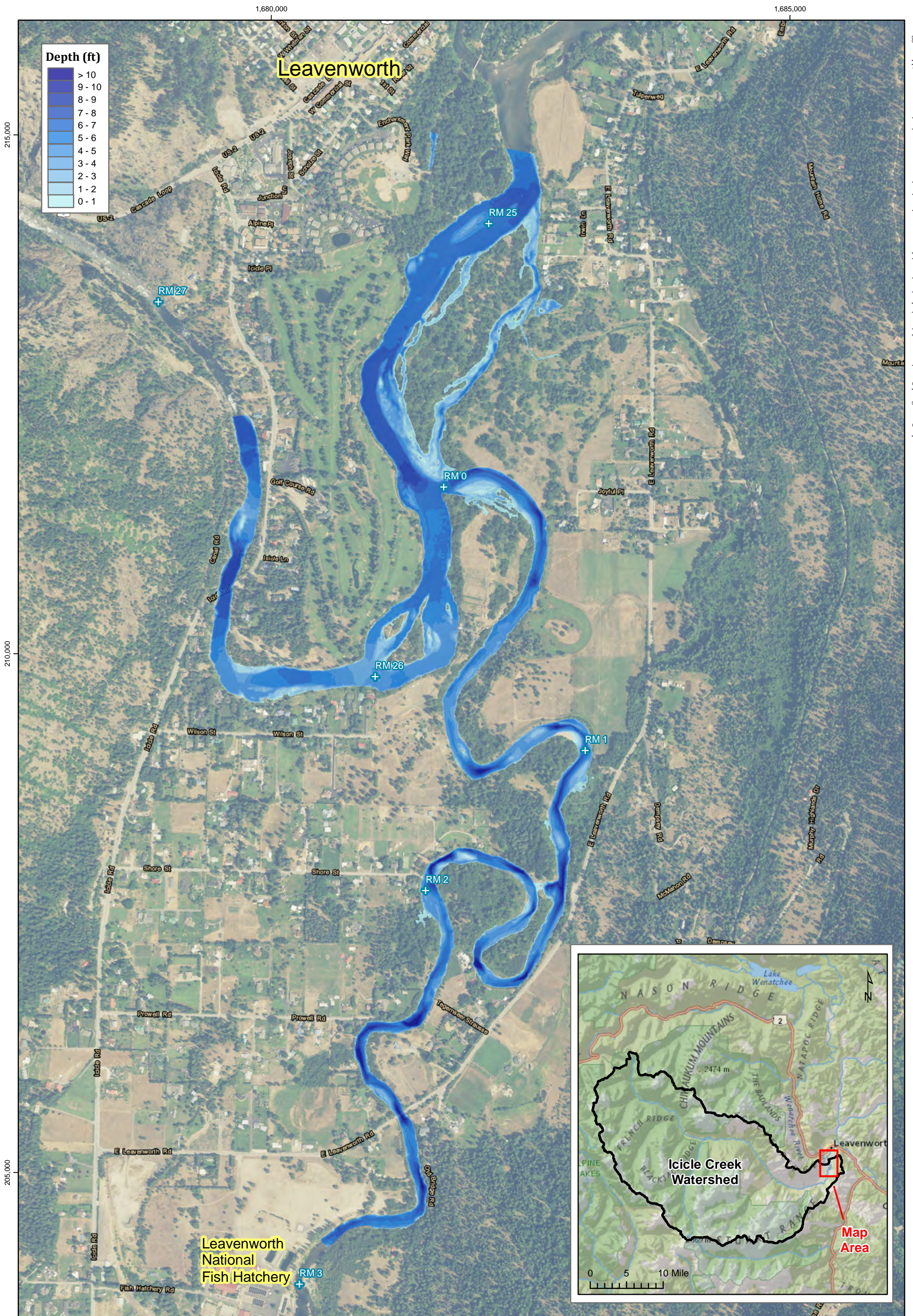
Icicle Creek Hydraulic Model Output - Spring Runoff (1830 cfs) Flow Depth
