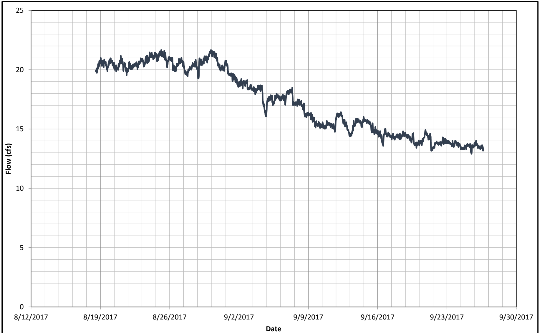
Figure C-4 Measured and Estimated Flows IID Division 3A Canal at ~ Station 725+00 IPID Comprehensive Water Conservation Plan
