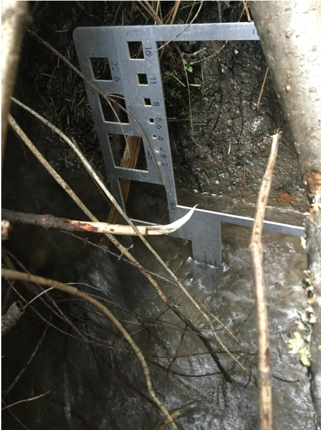
Figure 3. Evidence of bank seepage immediately downstream from Structure 5, on the left bank. Gravelometer for scale.
