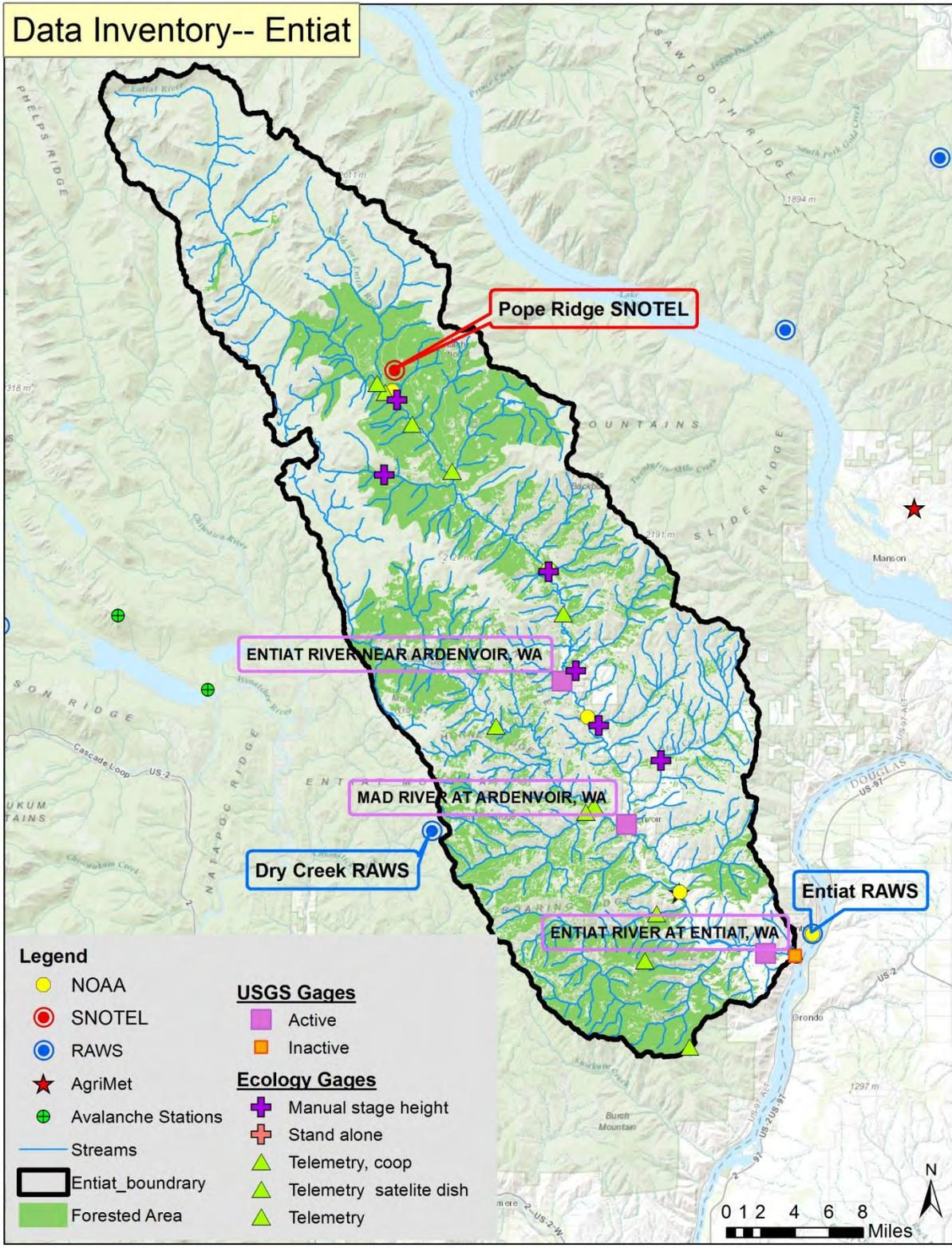
**Figure 24.** Available meteorological, snow, and streamflow monitoring stations in the Entiat subbasin along with areas that may be suitable for forest restoration.
