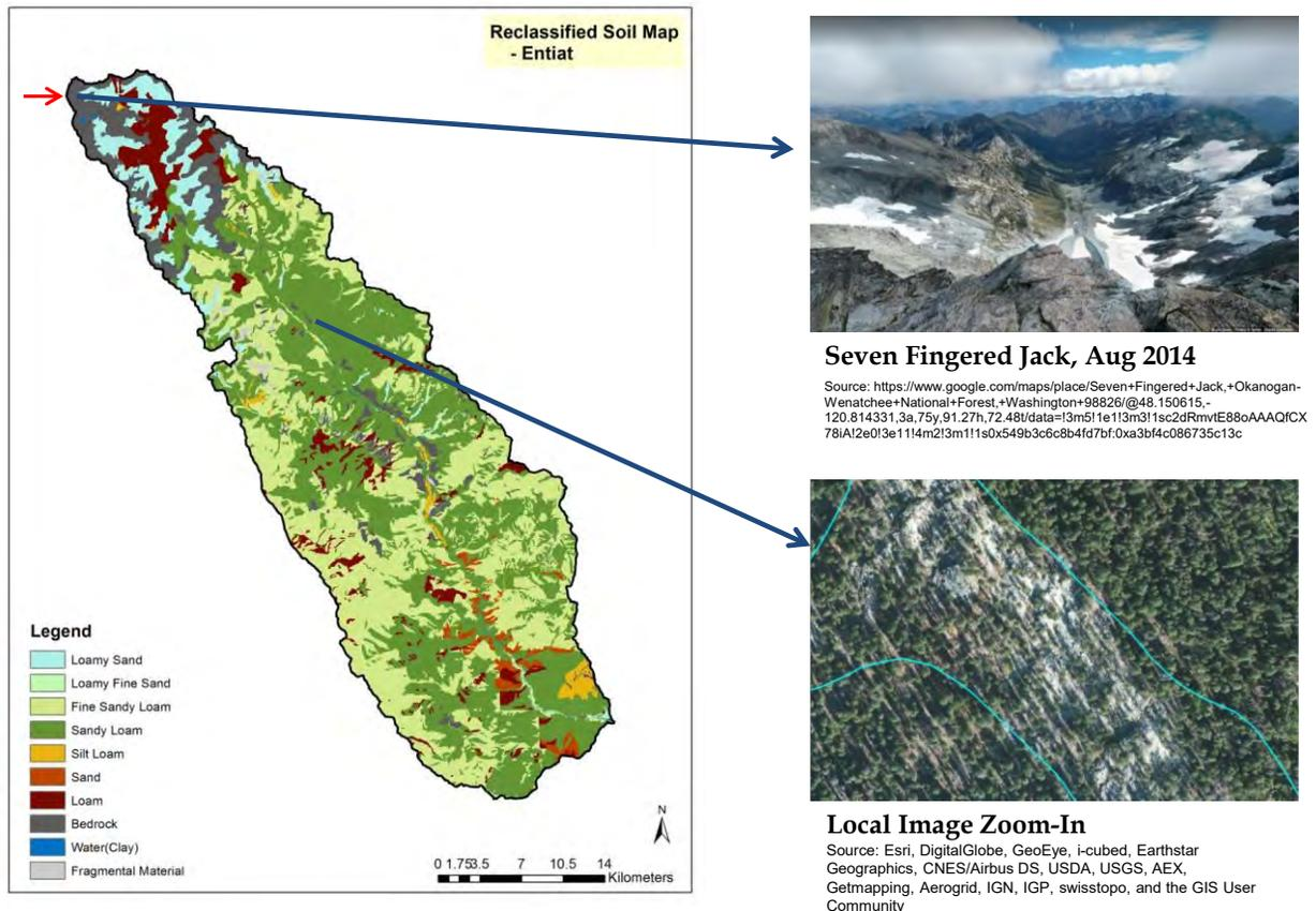
**Figure 5.** SSURGO-based soil texture classes for the Entiat subbasin (left). Areas of exposed bedrock are shown in the upper basin (upper-right image) as well as isolated bedrock exposure in forest (lower-right image).
