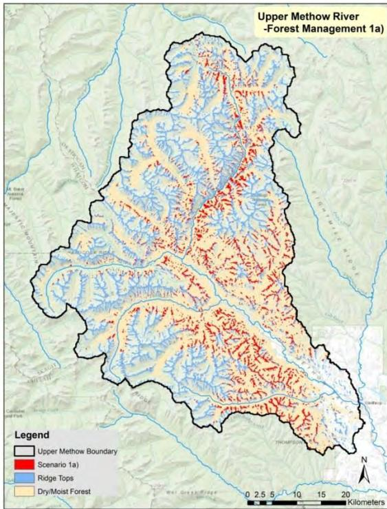
**Figure ES.3.** The Upper Methow watershed showing locations of forest restoration Scenario 1a with treatments on ridgetops in Dry/Moist forest types (red) where overstory fractional coverage was reduced to 30%.
