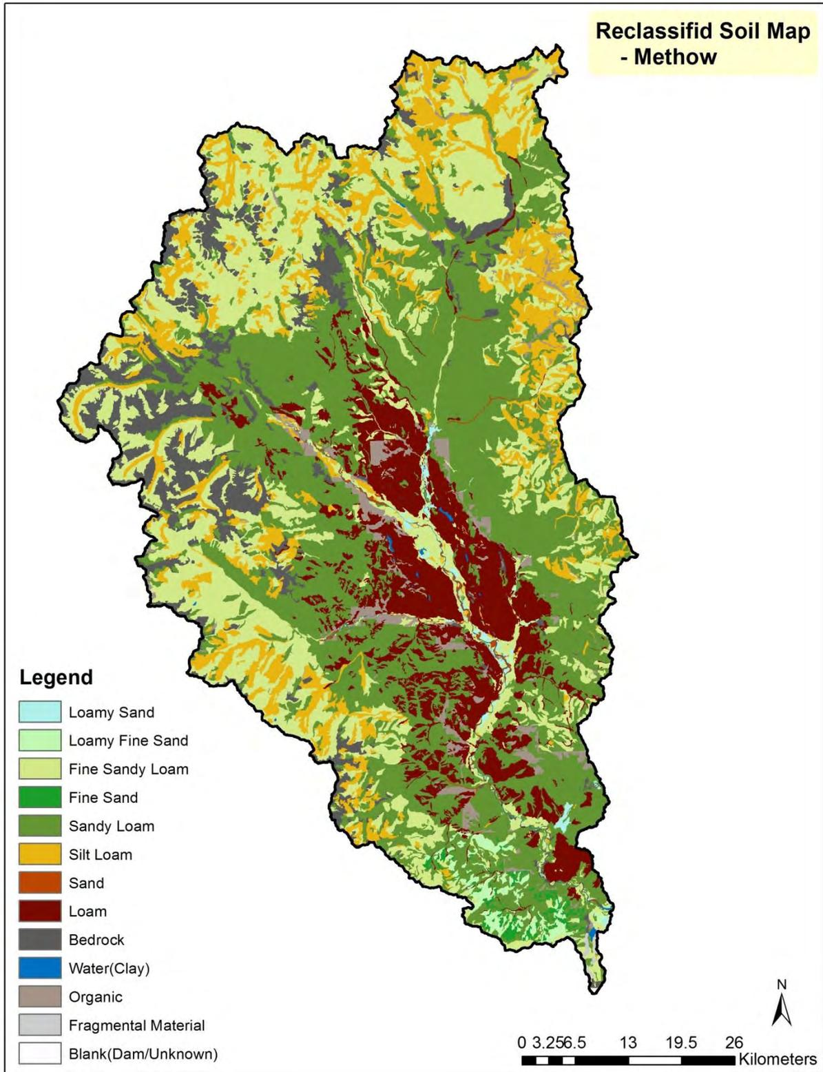
**Figure 61.** SSURGO-based soil texture classes for the Methow subbasin.
