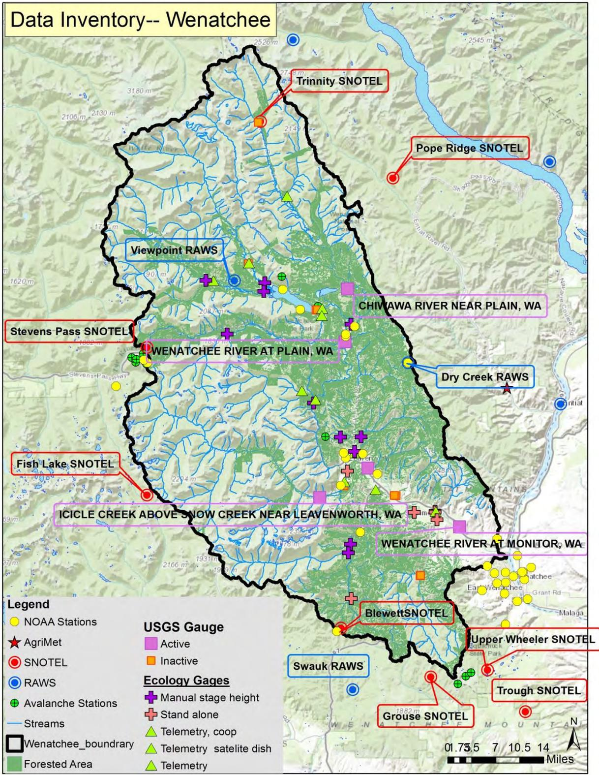
**Figure 42.** Available meteorological, snow, and streamflow monitoring data for stations in the Wenatchee subbasin along with areas that may be suitable for forest restoration.
