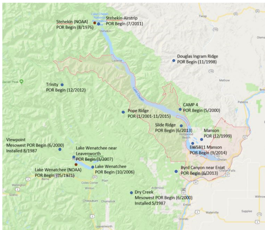
Figure 4. Rain gage locations in the vicinity of Slide Ridge site. Slide Ridge gage (center right of figure) is just north of the basin at the top of the ridge, with the best representation of rainfall. Manson gages are at lower elevations than Slide Ridge.
