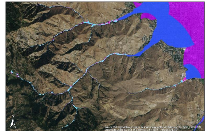
Legend FEMA DFIRM 100-Year Flood Boundary HAZUS and T1 Generated 100-Year Flood Boundary FEMA DFIRM 500-Year Flood Boundary HAZUS and T1 Generated 500-Year Flood Boundary 0 0.25 0.5 1 Miles
