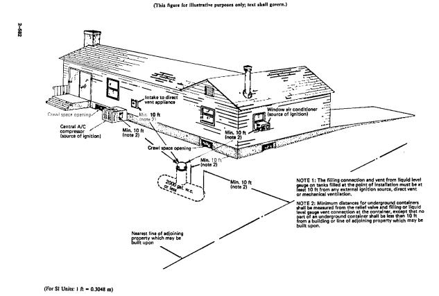
Figure I-3 Underground ASME Containers.
