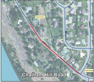
The current stormwater conveyance system in the West Eaglerock and Chatham Hill areas, needs to be improved to safely capture and convey runoff brought on by the short, intense summer rainstorms that often occur in the Wenatchee Valley. A hydrologic analysis completed in 2016 outlined specific upgrades to the stormwater system that would help minimize erosion and sediment
