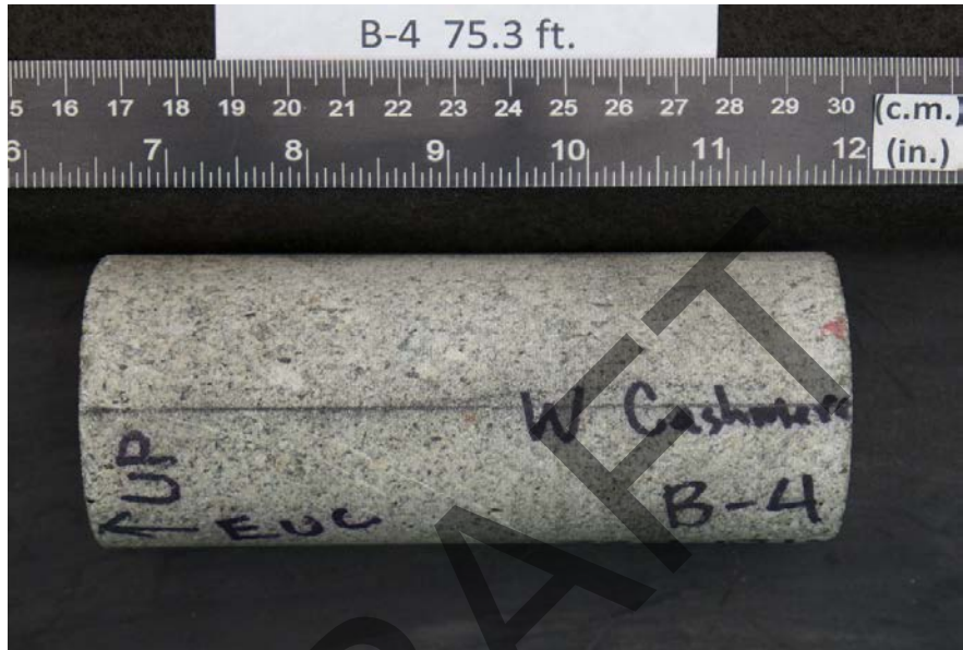
After cutting and grinding
