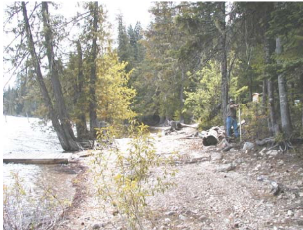
Photograph 5.2-3. Water line at Camp Zanika Beach approximates OHW Alternative while base of survey rod depicts approximate El. 1872.4. Water elevation on this date were approximately at OHW 1870.3.
