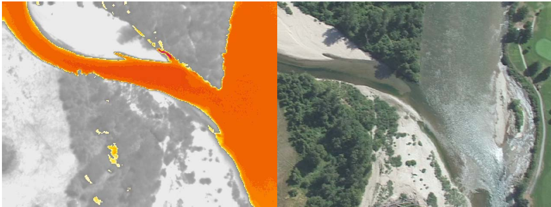
TIR/color video image pair showing the location of what appears to be a spring (16.5°C) on the left bank of Icicle Creek (17.4°C) just upstream of its confluence with Wenatchee River ( frame: Ice20018 ).
