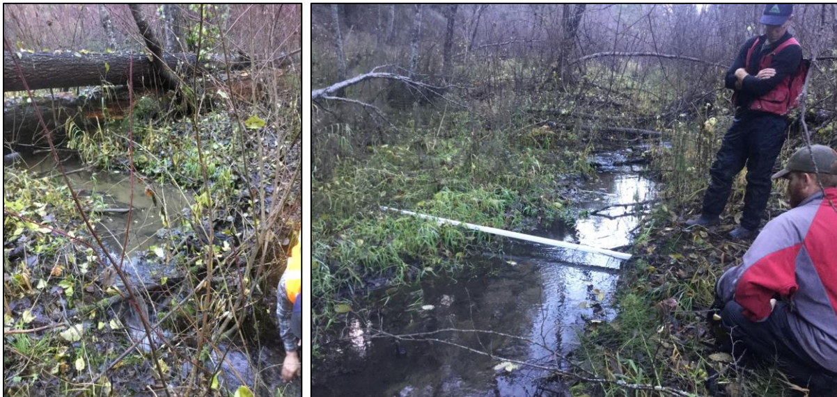
Figure 8. Photos of wetland reaches in Poison Canyon showing wood as the downstream hydraulic control (left) and shallow height (0.5-1') from water surface to bank (right).
