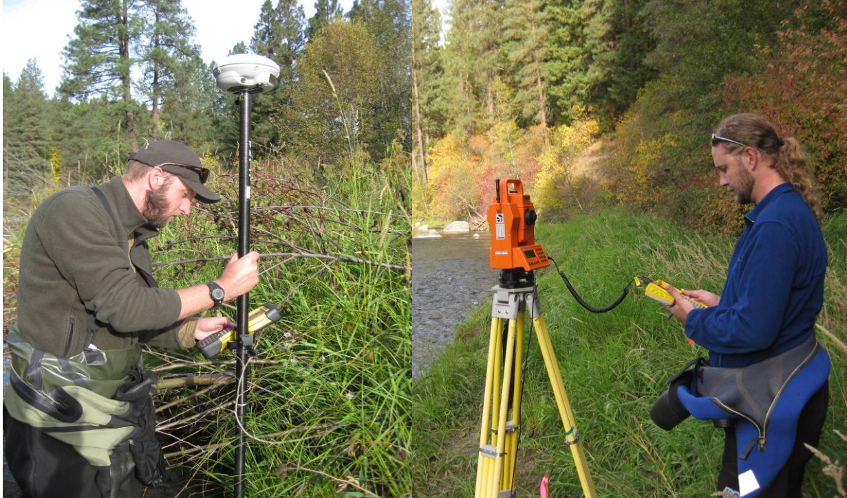
Figure 4. Survey grade RTK GPS (left) and total station (right) used to collect topographic data of the Icicle Creek historical channel.
