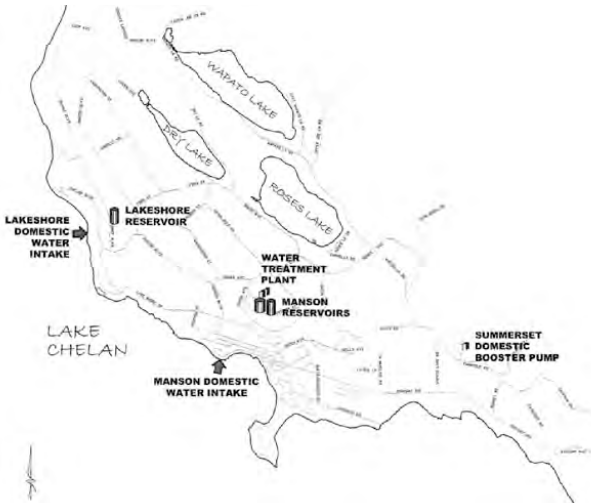
Figure 6.2 – Manson water/sewer treatment and distribution system
